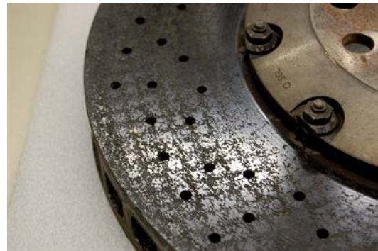
Brake disc surface exhibiting burnout
