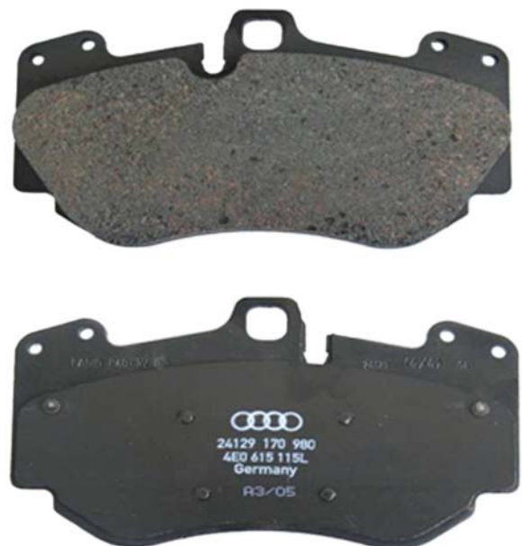
Organic brake pads for the ceramic brake
