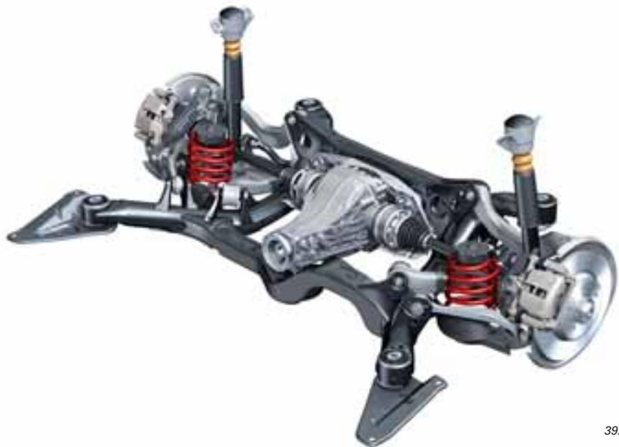
Rear axle of quattro models
