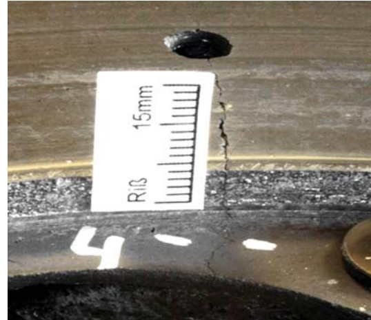
Critical interfacial crack propagation characteristic
