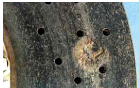
Chipping of the friction layer
