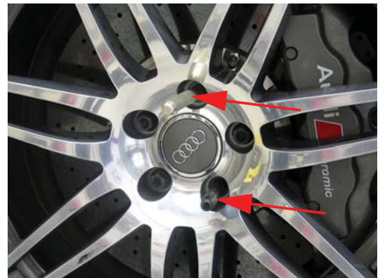
Screwed-in assembly drifts
