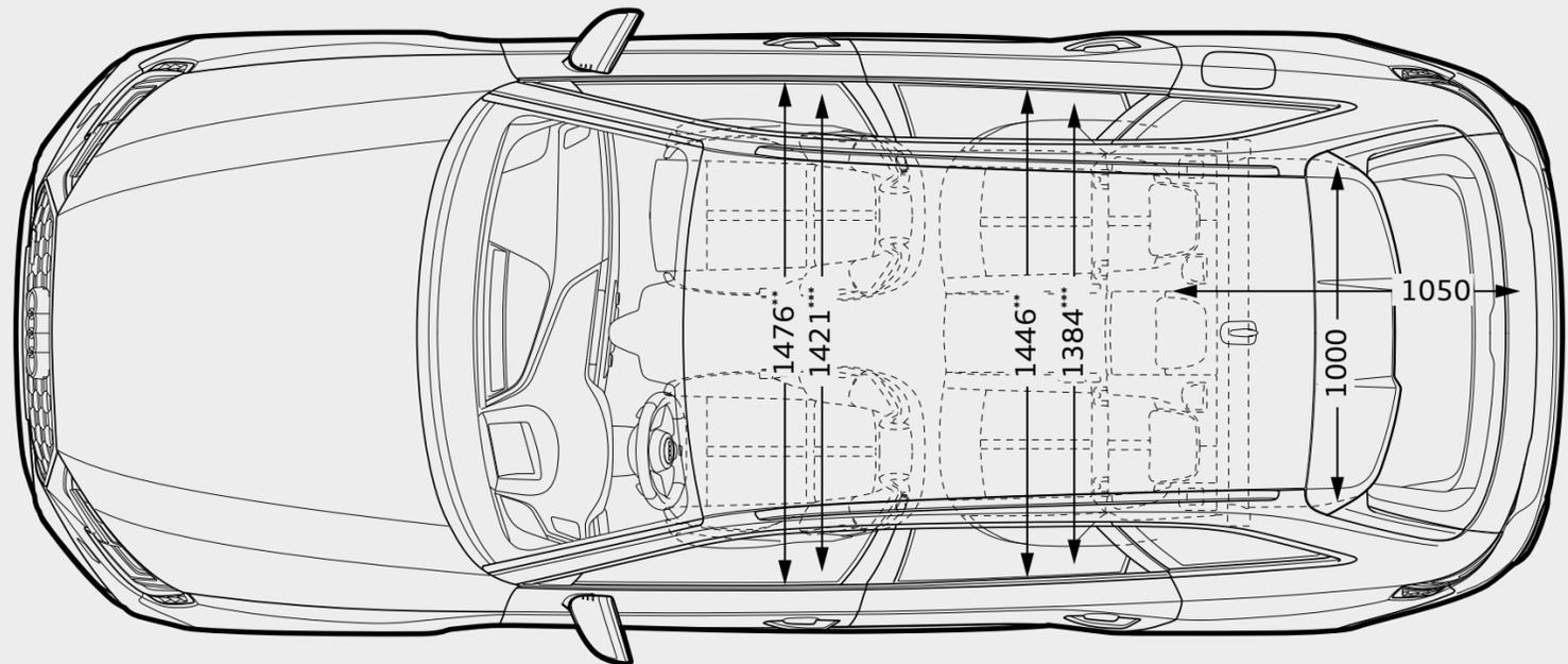
Dimensions in millimetres. Optional equipment may affect dimensions. Dimensions were measured with vehicle at unladen weight, ground clearance measured with vehicle carrying its maximum load. Turning circle approx. 11.7m.
