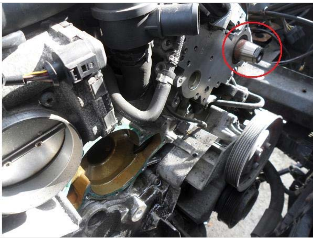
Thermostat housing now removed.
